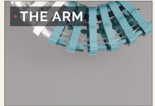
Seahorse-tail arm prototype, bending
